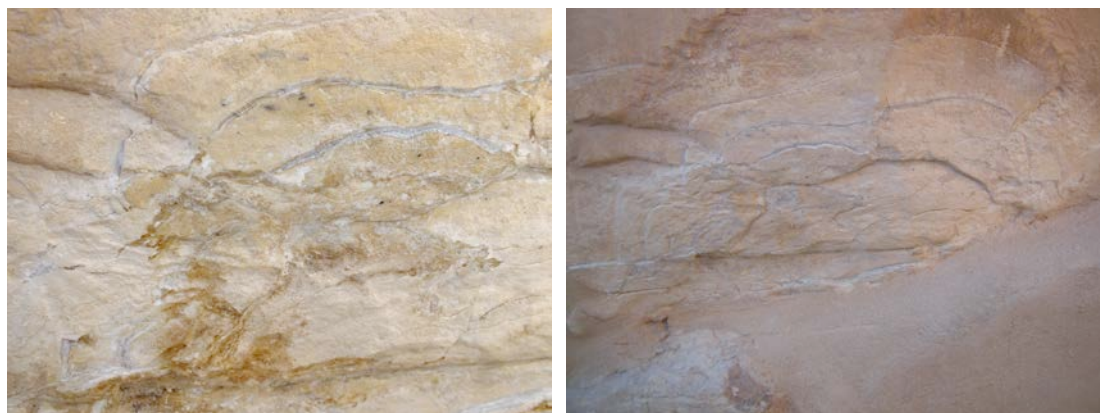
The surplus of old Araldite, before and after cleaning © Cnrs-Cfeetk/C. Bourse.
