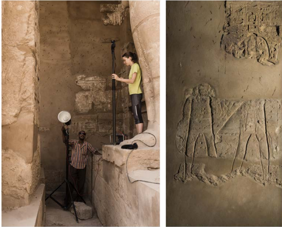
Left: Shooting in Ramses III temple using a pole and a flash; Right: Orthophoto obtained after images treatment with Photoscan and Photoshop. © CNRS-CFEETK/Ch. Wolff.
