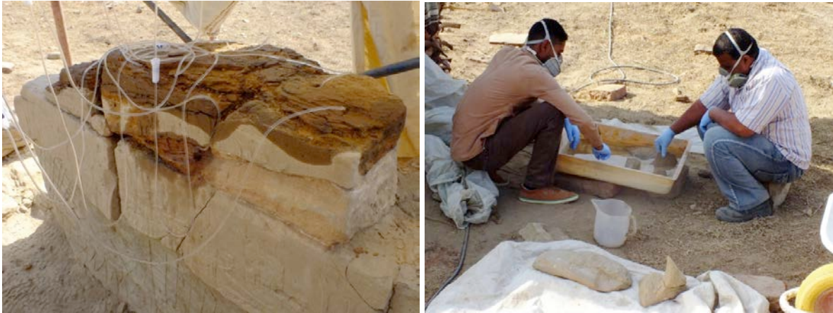
Two methods were used to silicate the blocks: infusion drips and baths © CNRS-CFEETK/C. Bourse.
